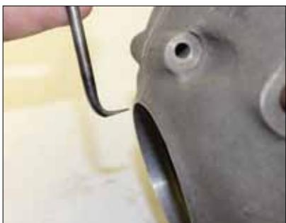
Fig. 12: Pick for extracting a propshaft seal.
