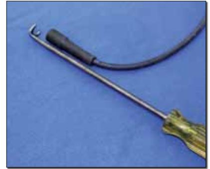
Fig. 11: Spark plug boot puller.
