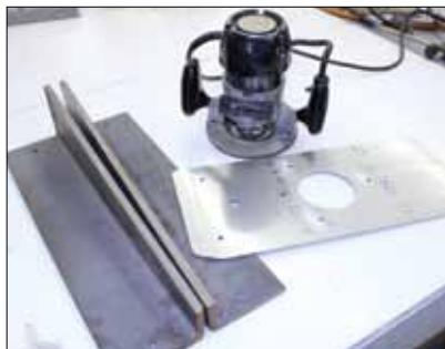
Fig. 19: Scarf guides milled from steel angle.
