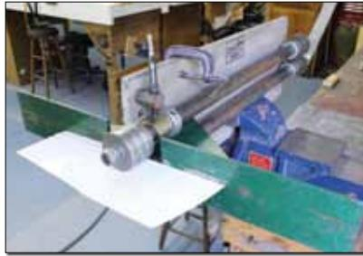
Fig. 3: Guide fence (green) added to bead roller.
