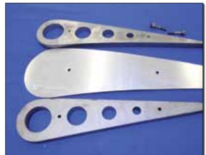
Fig. 20: Steel hammerforms and aluminum rib blank (center).
