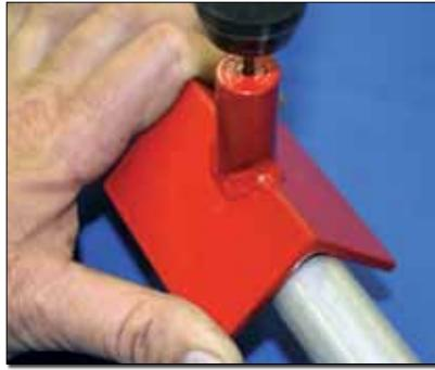
Fig. 16: Drill guide aligns paired, opposing holes.
