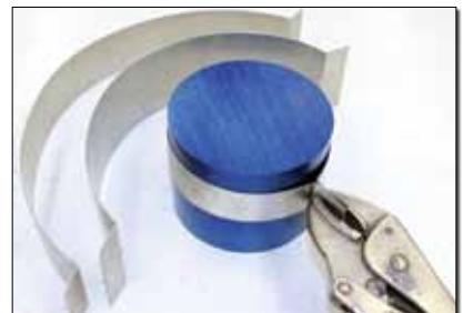
Fig. 8: Sheet metal band used as a ring compressor.
