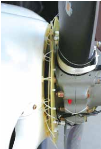
Signals from the strain gauges are collected in this circular module that houses a power supply, analog-to-digital converter and RF data transmitter. A small antenna is positioned on the cowling side.
