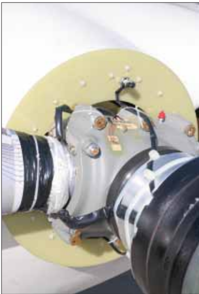
Signals from the strain gauges are collected in this circular module that houses a power supply, analog-to-digital converter and RF data transmitter. A small antenna is positioned on the cowling side.
