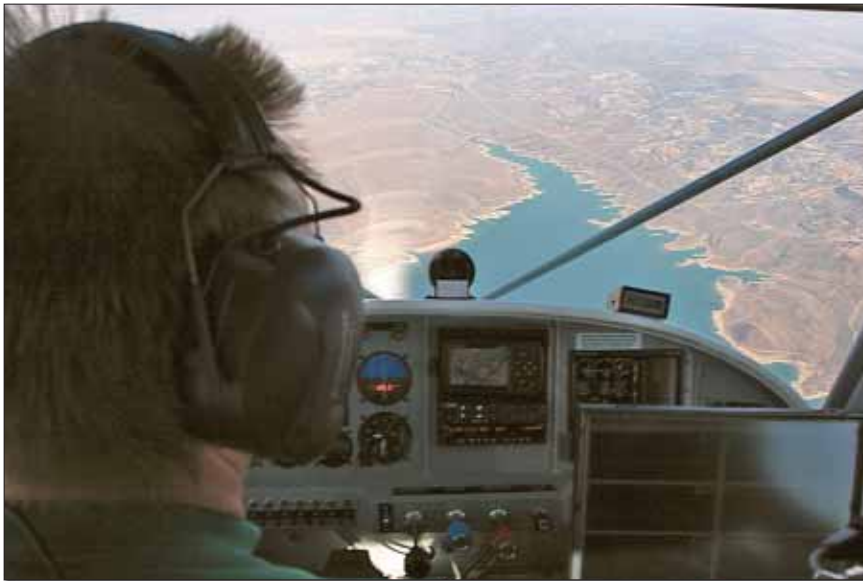
This is the view out the windshield during the gas-pressure test. It involves an idle-power pushover followed by a pitch-up to the stall. Fun!
