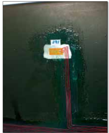
Tiny strain gauges are plastered all over the prop blade, shank and even buried in the hub. No stone is unturned.
