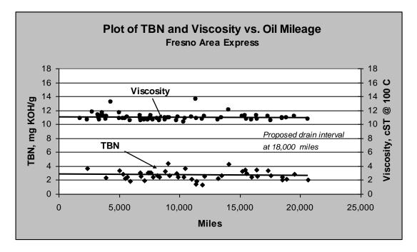
Figure 8. Plot of TBN and Viscosity vs. Mileage for FAX vehicles
