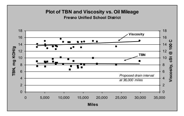
Figure 9. Plot of TBN and Viscosity vs. Mileage for FUSD vehicles
