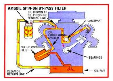
Figure 1. Typical Bypass Filter Installation (Diagram courtesy of Amsoil Corporation, Superior, Wis.)
