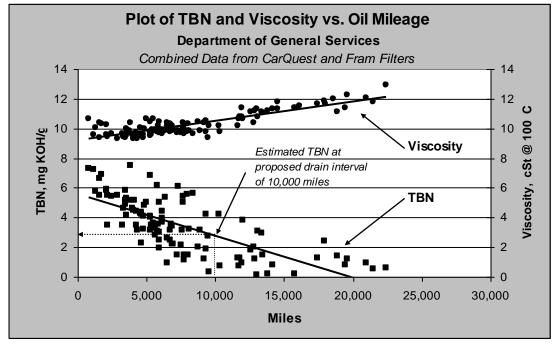
Figure 4. Plot of TBN and Viscosity vs. Mileage for DGS vehicles
